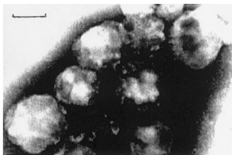
Figure 5 TEM photograph of polymer particles obtained by conventional seed emulsion polymerization, and employing preswelling of seed particles. The mixture of styrene monomer and SDS aqueous solution is treated by homogenizer at 4000 rpm for 20 min, and the PMMA seed latex is swollen by styrene monomer for 24 h before the seed emulsion polymerization. The weight ratio of monomer to seed particles is 1. The polymer particles obtained from conventional seed emulsion polymerization using APS as an initiator are stained with \text{RuO}_4 . The dark regions are polystyrene rich domains, and the lighter regions are PMMA rich domains. The scale is 100 nm.
